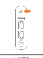
\* With the power of the product turned on, press this button with a fine-tipped object. RESET button Operation Press and hold for Reset the device setting to the default over approximately two seconds
